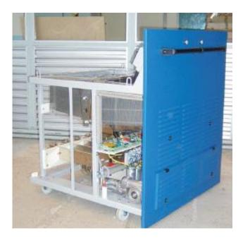
Two view on trolley cubicle converter – there are from back side - up good visible condensers of diode block and down contact head
