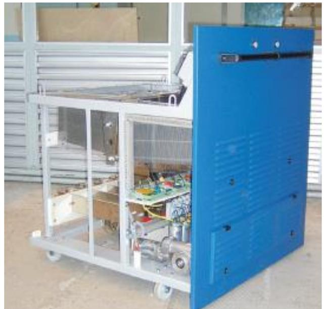
Two view on trolley cubicle converter – there are from back side - up good visible condensers of diode block and down contact head
